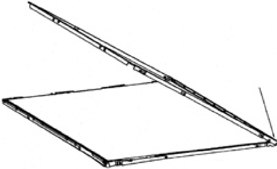
Figure 4-65 Replacing Sharp fluorescent lamp (SXGA+) (4)
