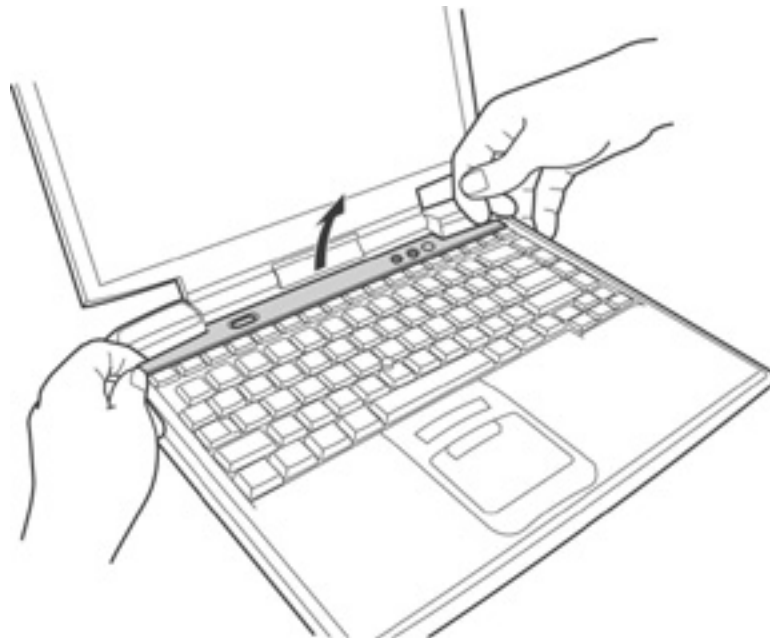
Figure 4-15 Removing the Keyboard brace
